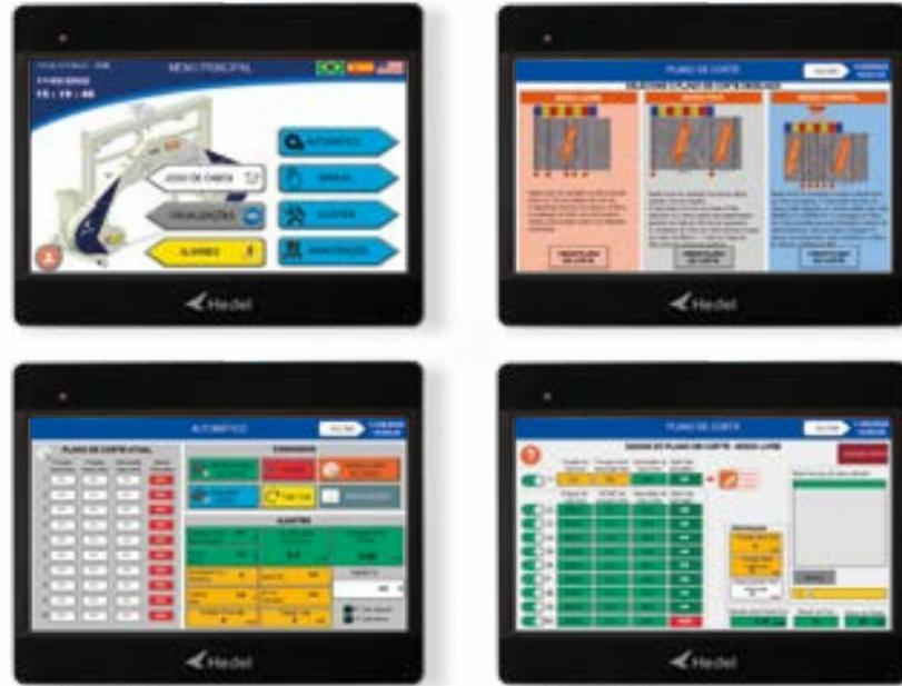
**IOT SYSTEM:** Developed in the industry 4.0 concept, through the cell phone it's possible to follow machine indicators in real time, from anywhere. Information such as: machine lifting, amperage, cutting time, time to complete the cutting and among other information.
