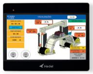
**IOT SYSTEM:** Developed following the Industry 4.0 concept; using your mobile phone it is possible to check indicators of the machine in real time from anywhere. Information such as: Machine lifting, amperage, cutting time, time to complete the cutting among other information. Feeding information to the panel the system informs service life of the wires, pearl wearing, provides a complete database allowing this way to create strategies to cut costs, increase production and improve the cutting.
